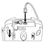
Place the telephone cord inside the molded channel on the bottom of the Base Unit.
